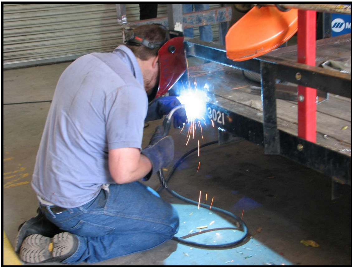
Trailer welding repair
