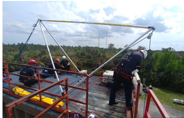
TRT setting up the Larkin frame on the roof of the county fire-training tower
