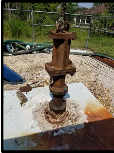
Vibratory Hammer used to drive pipe into the soil by vertical vibrations.
